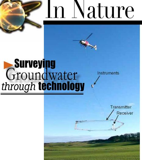
high-tech method has recently helped the NRD with needed groundwater monitoring.
