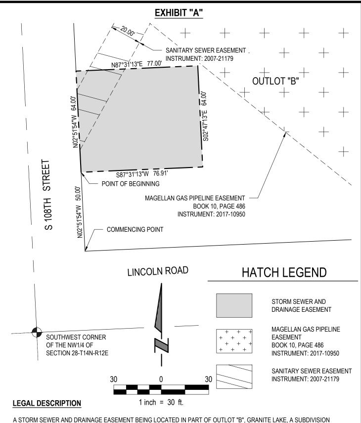
A STORM SEWER AND DRAINAGE EASEMENT BEING LOCATED IN PART OF OUTLOT "B", GRANITE LAKE, A SUBDIVISION LOCATED IN PART OF THE NE1/4 OF THE NW1/4, PART OF THE SE1/4 OF THE NW1/4, PART OF THE SW1/4 OF THE NW1/4 AND PART OF THE NW1/4 OF THE NW1/4, ALL LOCATED IN SECTION 28, TOWNSHIP 14 NORTH, RANGE 12 EAST OF THE 6TH P.M., SARPY COUNTY, NEBRASKA. MORE PARTICULARLY DESCRIBED AS FOLLOWS:
