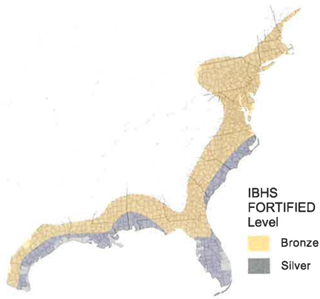
Figure 9. Maximum level of the IBHS FORTIFIED Home Hurricane design for new construction where the incremental benefit remains cost-effective.
