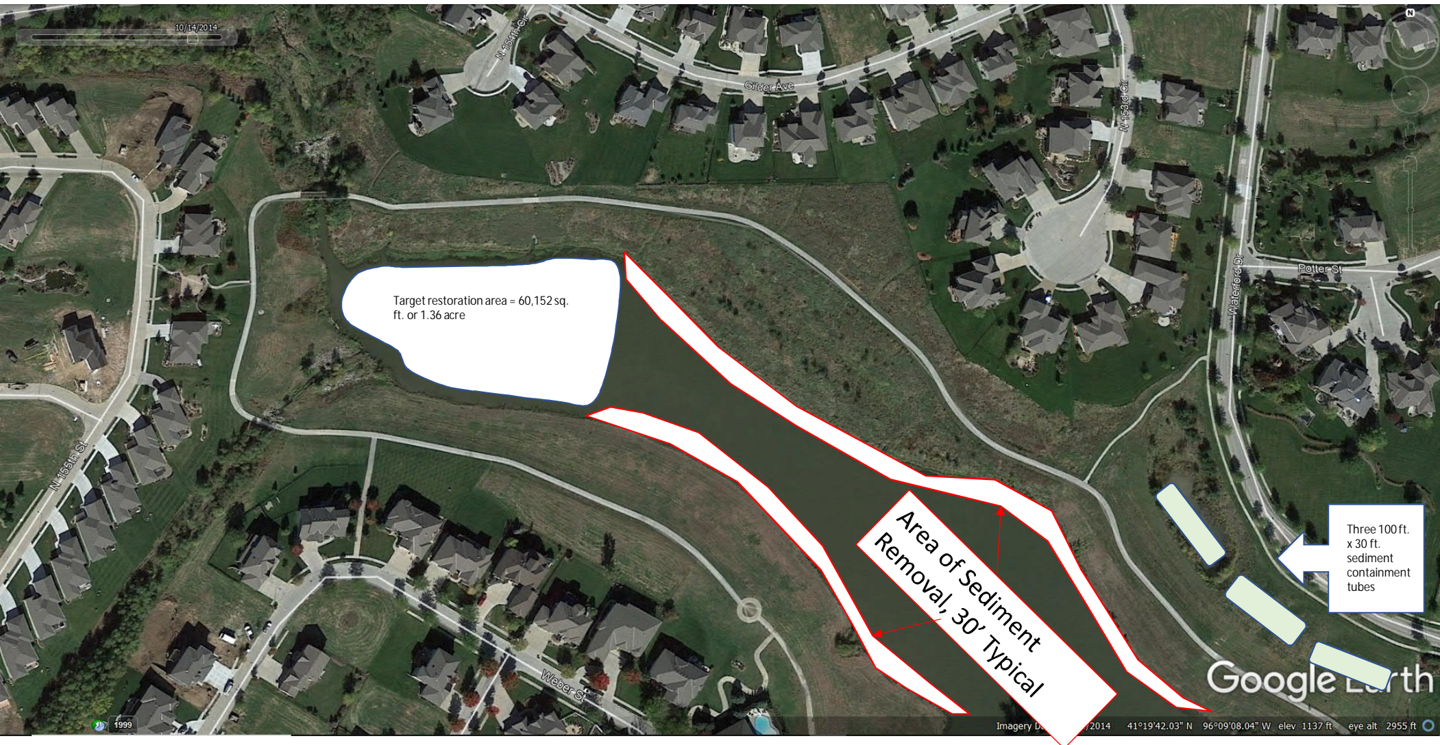
Waterford Lake retention pond, sketch for target area 'A' on the northwest end of the pond. This area measures approximately 60,152 sq. feet or 1.38 surface acre. This area is holding approximately 2.5 feet of organic sediment with some aquatic weeds. We estimate the hydraulic removal of 556 cubic yards of dewatered organic sediment. It will take three 100 ft. x 35 ft. sediment containment tubes to hold and dewater the material.
