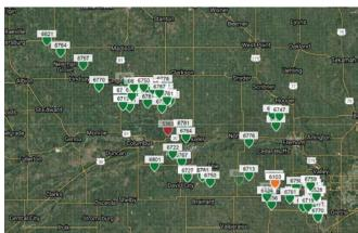
There is additional need within our NRD to expand our continuous groundwater monitoring sites between the Platte and Elkhorn Rivers. This expansion would focus on having a cross section of monitoring sites that extends north to south, from Arlington to the Linoma beach area. The location of these proposed nine additional monitoring sites as well as the six existing groundwater monitoring sites is shown in Figure 1 attached.
