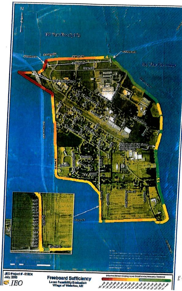
The Waterloo levee improvement project proposes levee modifications to accredit the levee to Federal Emergency Management Agency (FEMA) standards and continue to provide 100 year flood protection for the residents of Waterloo. The Waterloo levee is a ring levee which surrounds the Village of Waterloo and it is entirely in their jurisdiction. The estimated construction costs for the levee improvements are approximately \$4 million dollars.
