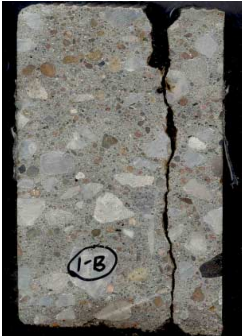
Figure 1. Scanned image of section through Core 1-B showing routed crack with sealer and full-depth view of crack. Note the darkened paste zone adjacent to the bottom, indicating water loss into the base material while the mix was still plastic.
