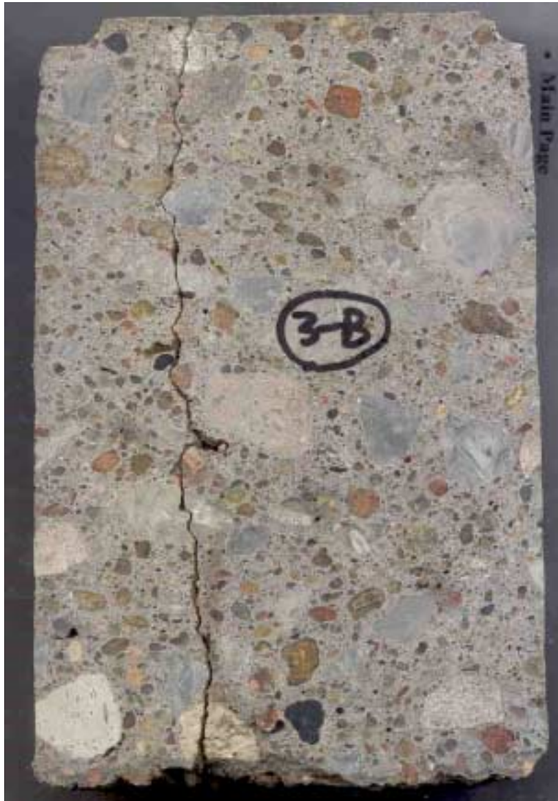
Figure 2. Full-depth crack in Core 3-B. The cracks pass through limestone coarse aggregates and some of the siliceous granitic gravel particles.
